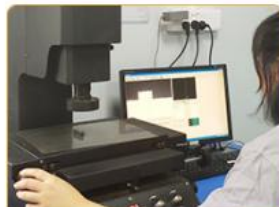
8.FQC for Size and Mechanical properties
