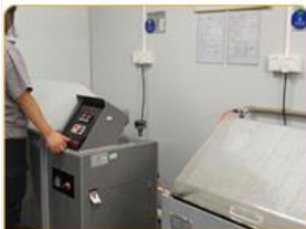
7.Salt spray test
