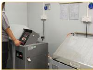
7.Salt spray test
