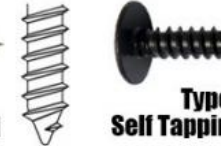
Type A Self Tapping Thread
